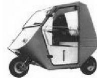
The first license-free cars, which came on the market in the 1970s, were one- or two-passenger, three-wheel car body-encased mopeds fitted with a noisy, low performance, petrol-powered dual-stroke 50cc engine. They had to weigh as little as possible, have a light frame and only the strict minimum of equipment (no heating, no boot, and sometimes no lateral windows or doors), to facilitate their smooth integration into traffic. Total authorised weight was 200kg.
