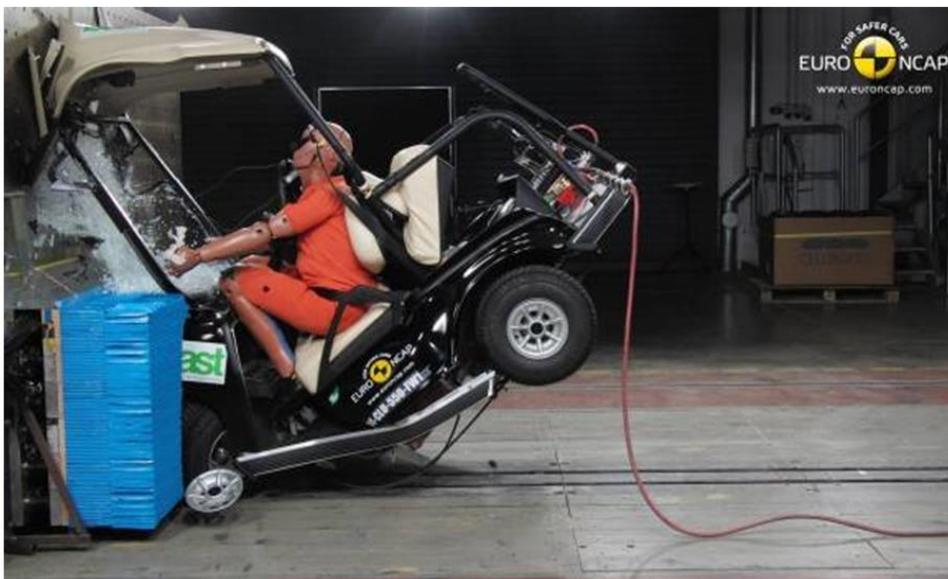
**Figure 3.** A light quadricycle, a golf cart fared really badly in a crash test (EURO NCAP courtesy)
